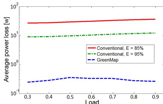
Figure 4: GreenMap reduces power conversion loss from the conventional architecture by two orders of magnitude.
