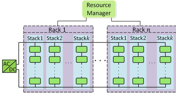
Figure 1: Data center with series-connected stacks.
