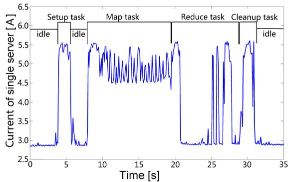
Figure 2: Current consumption of a word-count job with one map task and one reduce task.
